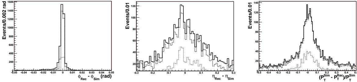
Figure 10: From left to right resolutions of  $\phi$ ,  $\eta$ , and the transverse momentum relative resolution. Resolutions are shown for all the tracks (solid), for tracks with hits at least in three layers (dashed) and for tracks that have hits in four layers (dotted).
