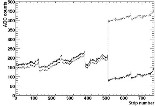
Figure 32: Module with high pedestals on last two APVs. Pedestals are shown for run 20391 (solid) and run 20400 (dashed).
