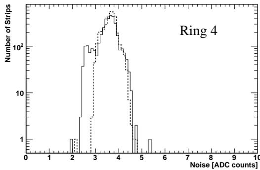
Figure 38: Tick mark height calibrated (dotted) and uncalibrated (solid) noise of ring 4 modules.
