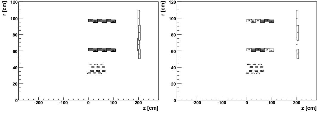
Figure 5: The left plots shows an overview of the inner seed rings (light grey) and outer seed rings (dark grey) as defined for the Road Search algorithm. The right plot shows the road of a possible cosmic ray track.
