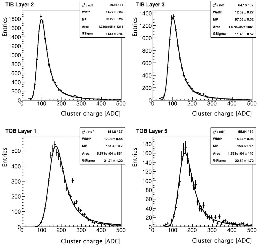
Figure 58: Cluster charge for TIB and TOB modules at  $B = 0$  T. The cluster charge is proportional to the detector thickness: nominally  $320 \mu\text{m}$  for TIB and  $500 \mu\text{m}$  for TOB, though in both cases the active sensor thickness is 20-30  $\mu\text{m}$  less.
