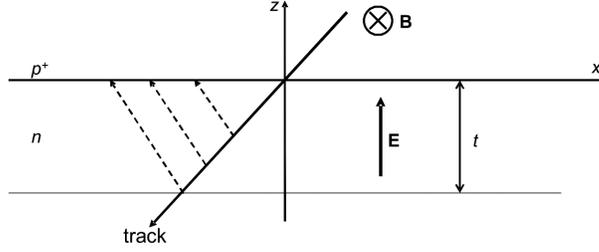
Figure 77: Lorentz drift in the microstrips silicon sensors.
