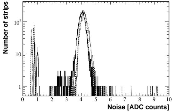
Figure 27: TOB Layer 1 tick mark height calibrated strip noise distribution for three pedestal runs
