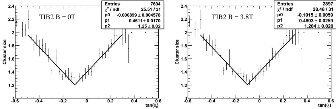
Figure 78: Cluster size versus incident angle in TIB Layer 2 for (a) no B field and (b) 3.8 T. The difference among the minima corresponds to the Lorentz angle.
